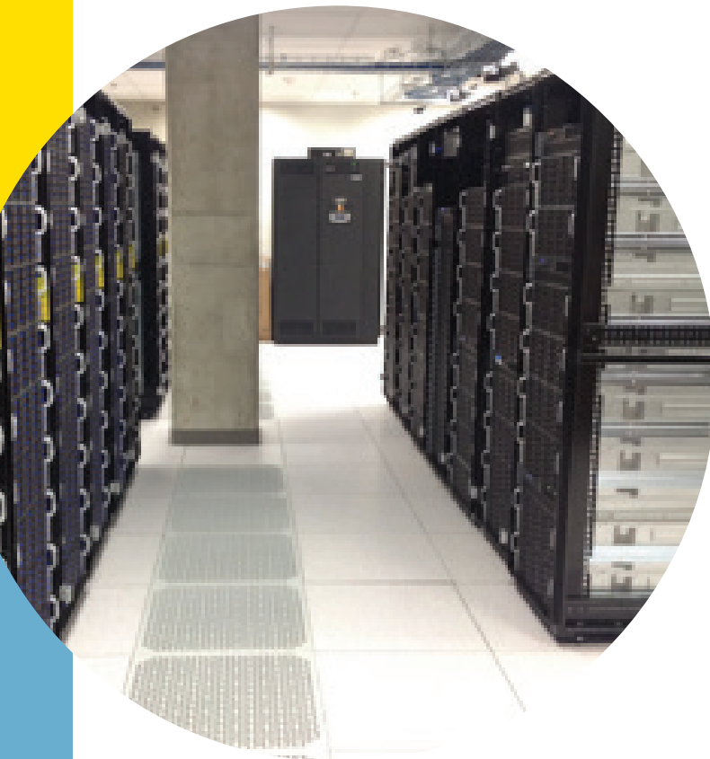
Figure 4: The JHU-based Data-Scope, with its 10PB of storage and 0.5Tbytes/sec I/O performance.
