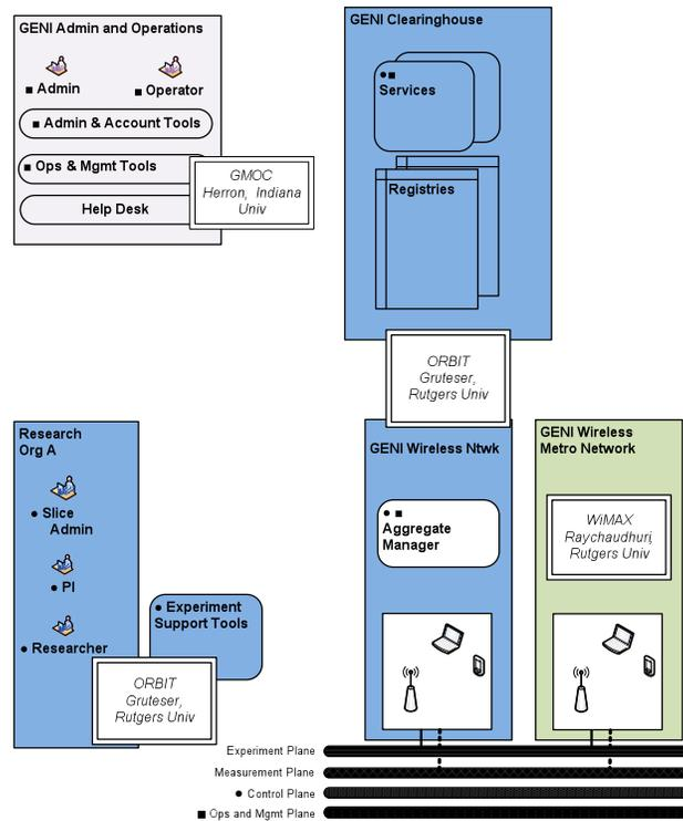
Figure 5-5. Cluster E utilizing “ORBIT” Control Framework
