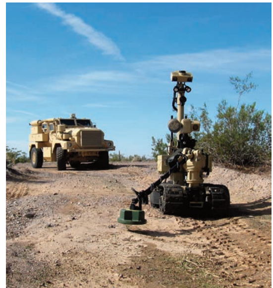
The Automated Mine Detection System (AMDS), developed by Carnegie Robotics, LLC, searches for landmines and IEDs.
