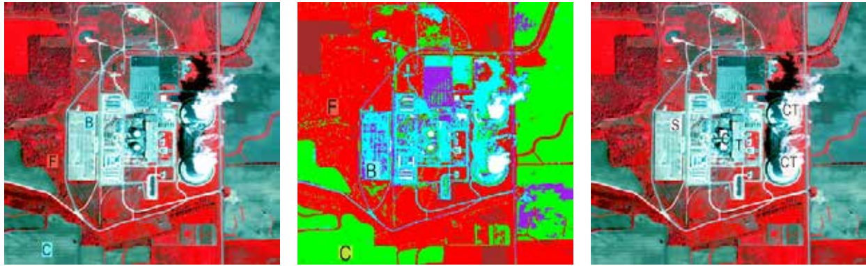
(a) FCC Image with Thematic class labels (B-Buildings, C-Crop, F-Forest) (b) Thematic Classified Image (Buildings, C-Crop, F-Forest) (c) FCC Image with Semantic Labels (S-Switch Yard, C-Containment Building, T-Turbine Generator, CT-Cooling Tower)
