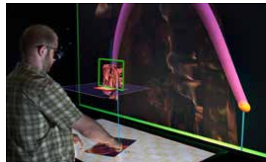
Figure 3: Designing medical devices in a virtual heart. Touch gestures are used to investigate a 3D heart model created from imaging data. Video: http://ivlab.cs.umn.edu/generated/pub-Coffey-2011-InteractiveSliceWIM.php
