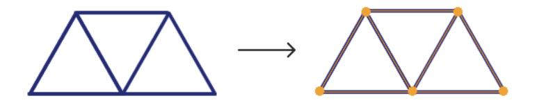
Use a shortest path algorithm to find the smallest possible polygons.
